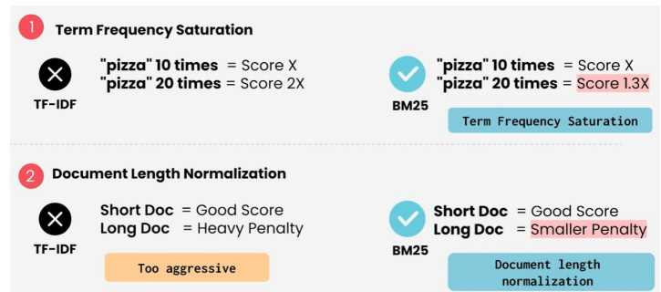
Figure: BM25 improves upon TF-IDF by applying term frequency saturation (reducing the weight of repeated terms) and balanced document length normalization (avoiding overly harsh penalties on longer documents).
